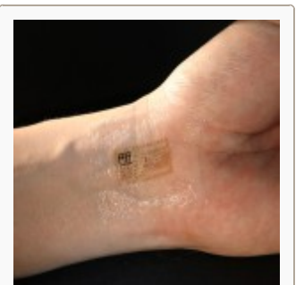
This isn't an ordinary temporary tattoo. This transparent device can measure a wearer's blood flow, muscle movement, electrical signals — and wirelessly send that information to a computer. Credit: Image courtesy of John A. Rogers
